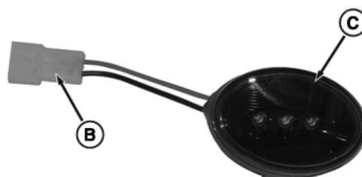
Remove Bulb From Retaining Ring
